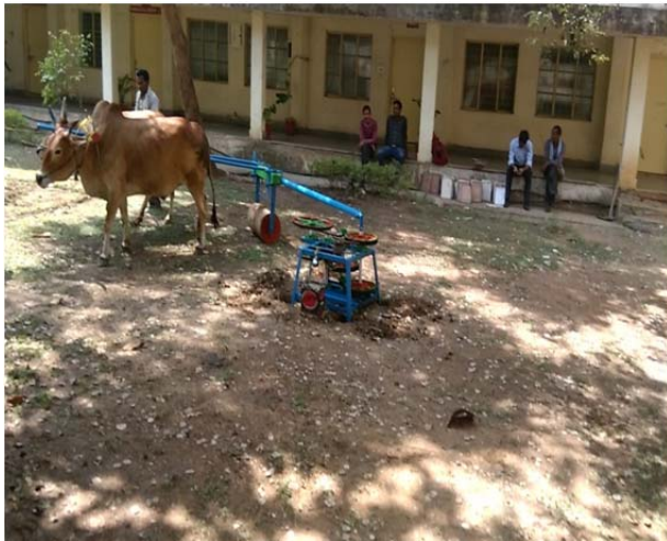
Fig. 3: Mechanical device for generating electric power using animal power.
